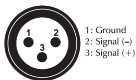
DMX-input XLR mounting-plug:
