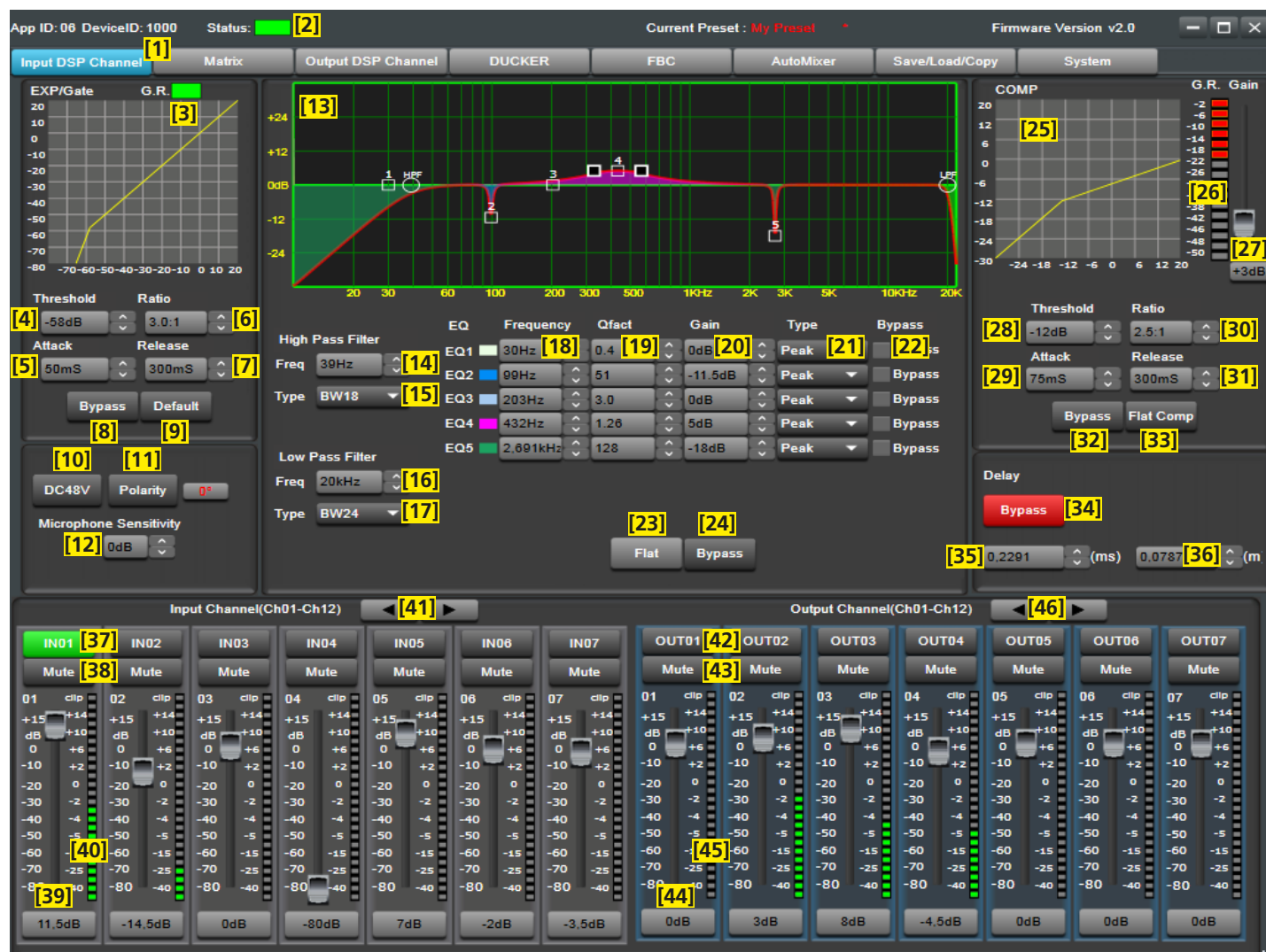
Fig. 20 View "Input DSP Channel"
